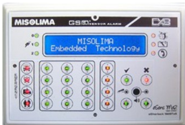
MISOLIMA eSherlock with static touch panel is the main home automation and security unit. It is based on GSM, USB or Wi-Fi communications. It uses the latest embedded technologies with DOLLx8.
